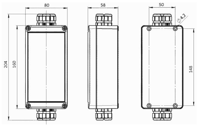
**Fastening holes** 4x clearance holes Ø4.2mm
