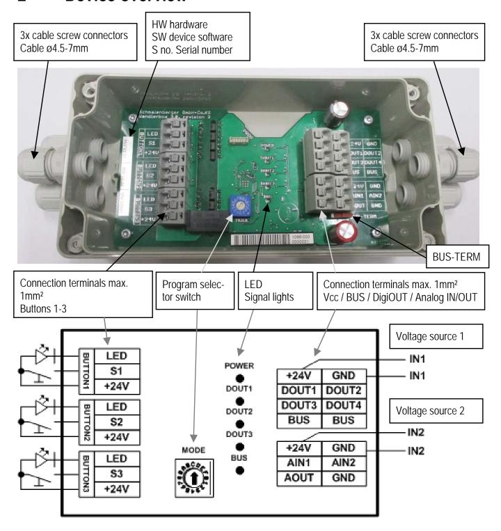
BUS-TERM Terminating resistor for bus system
